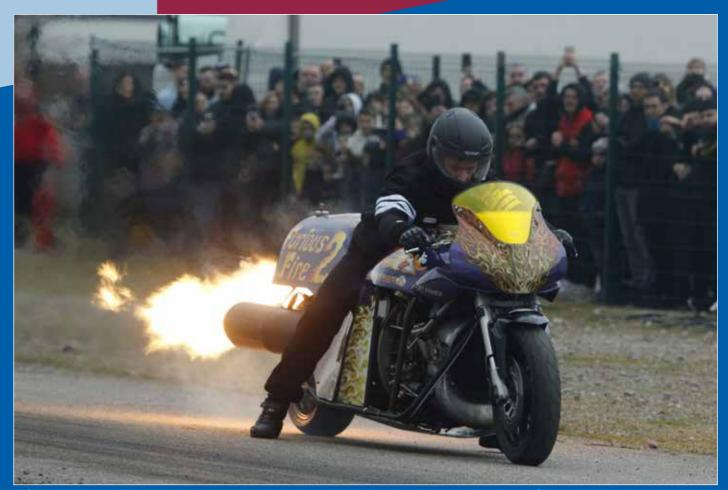
TOP: "Furious Fire" is the two-wheeled Jet-vehicle in the huge collection of Donald Pottiers garage: The custom-built motorcycle frame also hosts a Fogua "Magister" Marboré II jet-engine. BOTTOM: The afterburner is custom made and not original part of the original Jet trainer and acrobatic aircraft engine! At night or dusk a spectacular show finale.
