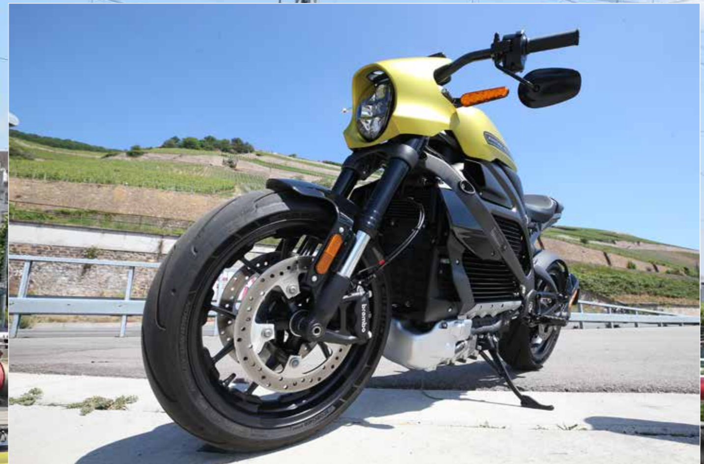
The look is deceiving: Battery and equipment carry some weight: 251 kg!
