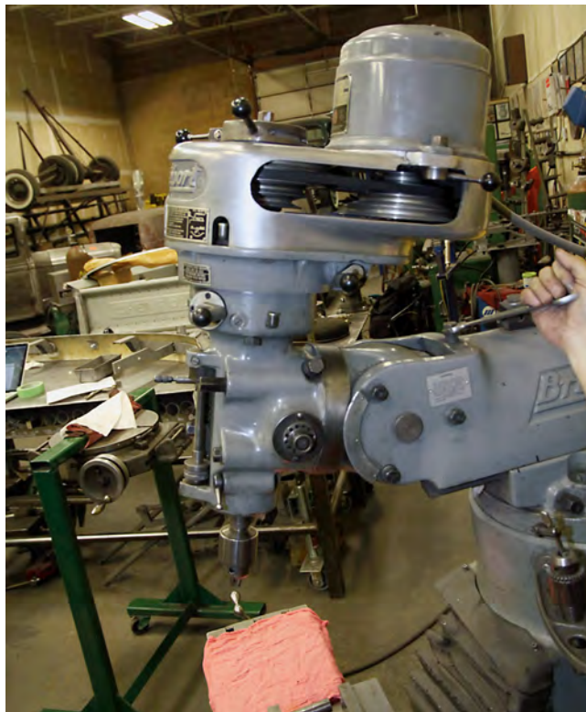
4) ... and use the adjustment (note Kurt's hand) to tilt the head as shown.
