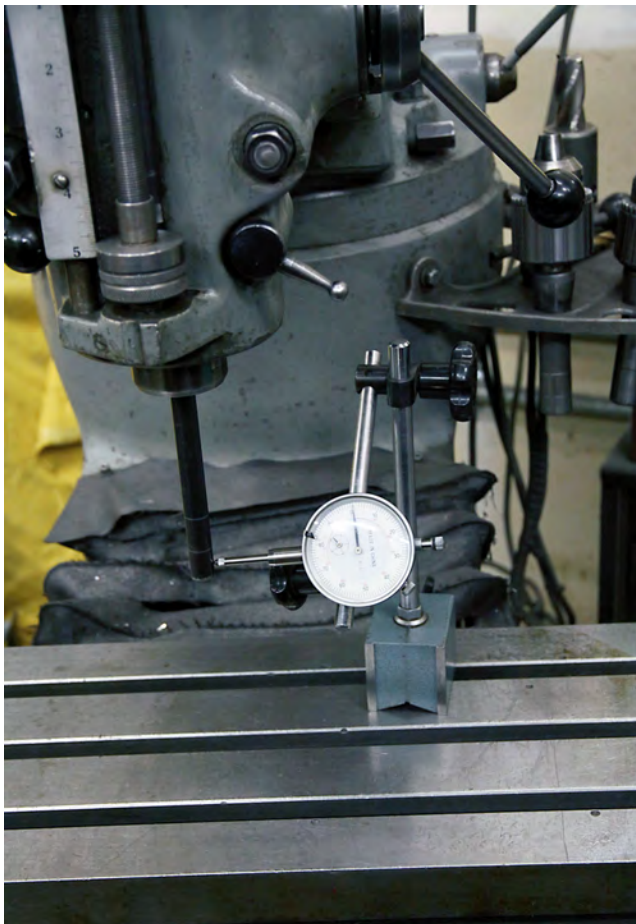
2) ... and the collet mounted in the mill, with the indecol and dial indicator set up as shown.
