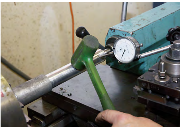
If a piece of work is taken out of the lathe, then reinstalled, it needs to be indicated with the dial indicator as shown. Sometimes a tap from a soft hammer is all that's required to bring it in line.
