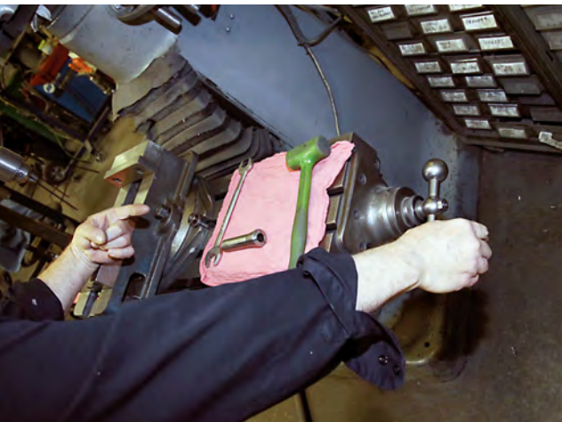
The table can be moved along the x axis (to the left and right) with the crank handle as shown.
