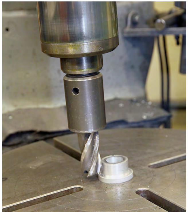
Center the table under the quill, add one end mill and you can make a step in the work, as shown, just by rotating the table as the end mill spins.
