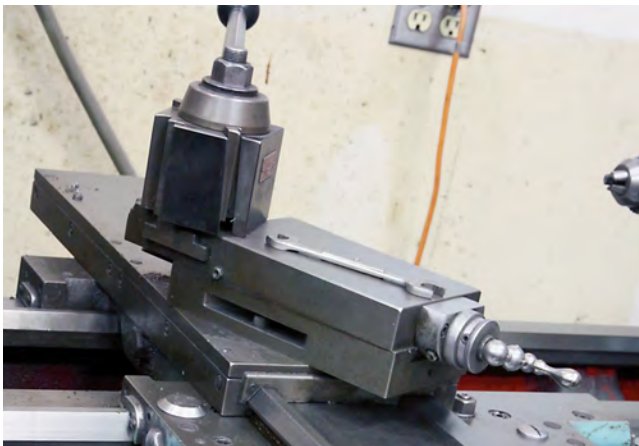
The Aloris tool holder does more than just hold the tool. Loosen two nuts and the mechanism rotates.
