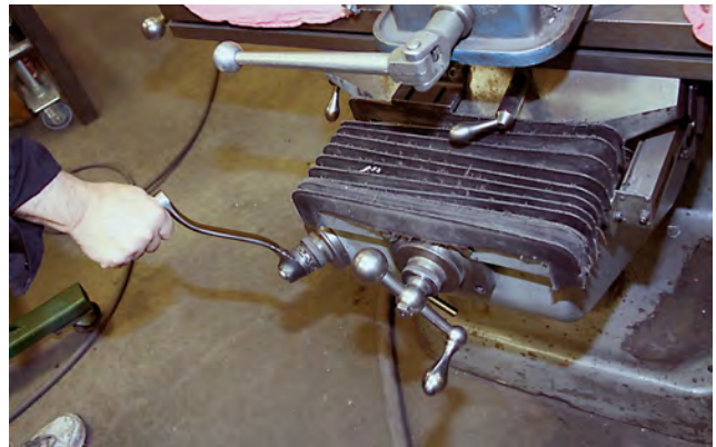
The third handle, shown here, moves the table along the z axis, (up and down).
