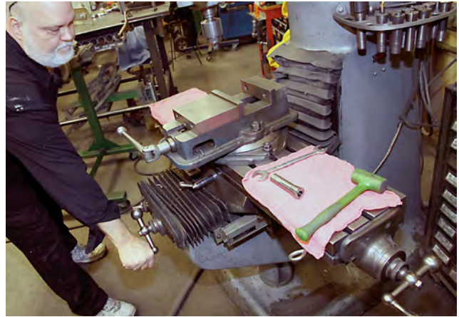
Moving the table along the y axis (closer or farther away from you) is done with the handle on the front of the machine.
