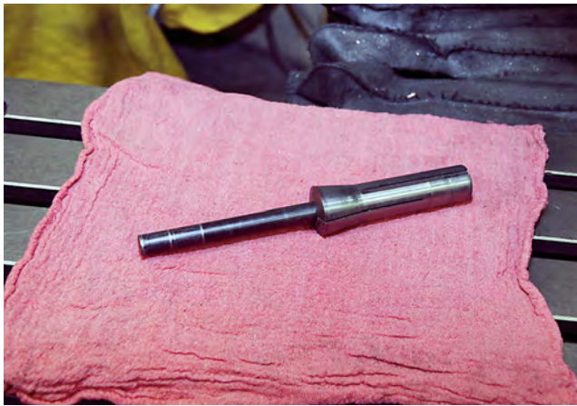
1) There is a simpler way to indicate the table. This Plan B, which starts with a piece of perfectly straight drill rod mounted in the collet...
