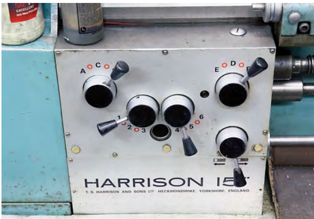
The lower levers control the speed and direction of the power feed.
