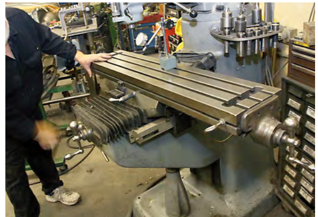
4) Now, use the big crank handle on the front of the mill to move the table up (on the z axis).
