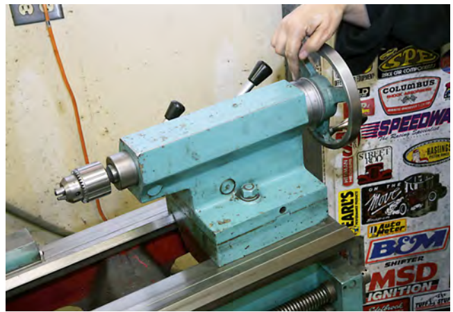
The tailstock can be equipped with a chuck for a drill bit as seen here, or more often, a shaft with a tapered end used as a support for the work.
