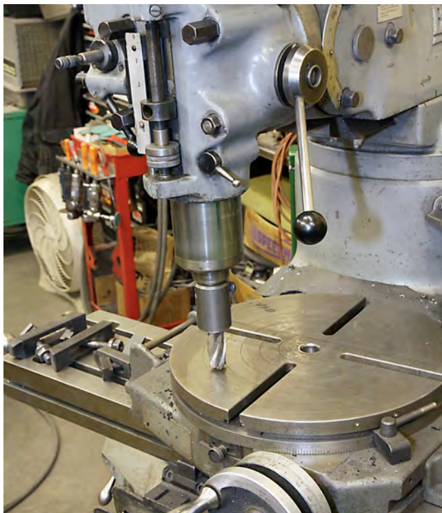
Locate the rotary table mounted off-center relative to the centerline of the quill, and the possibilities are almost endless.
