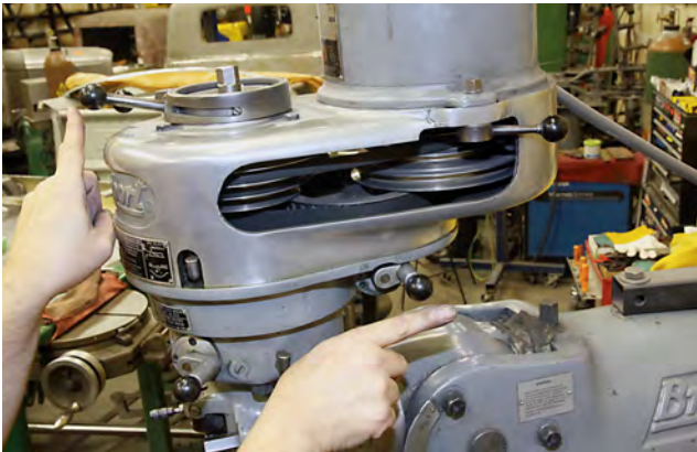
Changing from hi to low range is done by moving the two levers shown here, together is low, apart is hi. When going to hi range it's necessary to spin the chuck so you know the gears are engaged.
