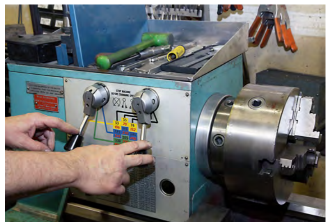
Not all lathes are the same, this Harris lathe uses the levers seen here to change the speed of the spindle.
