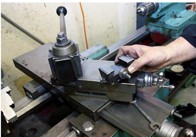
The part of the tool holder that actually holds the tool or can be popped off quickly by just...
