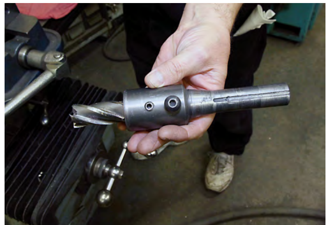
Close up shows a collet holding a 4-flute end mill. The taper matches the female taper of the quill, pulling the collet up into position with the drawbar tightens the collet's grip on the tool.
