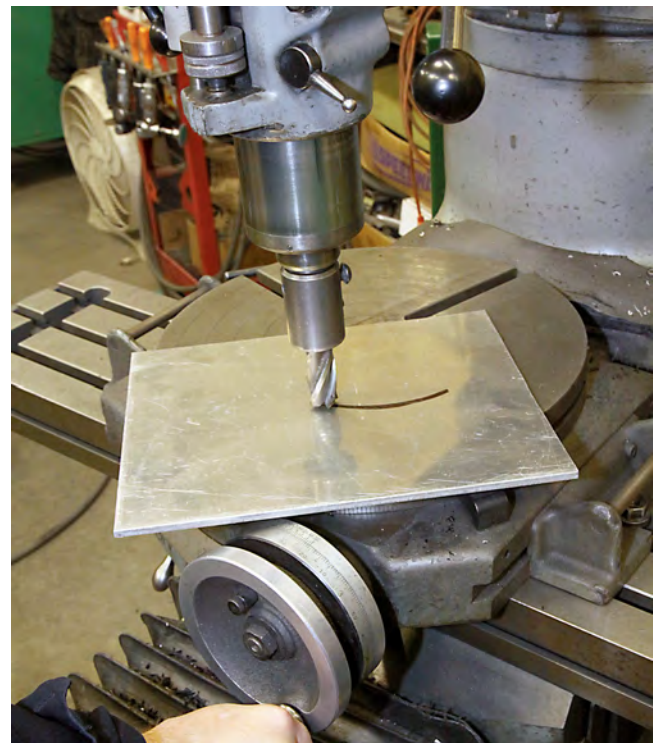
The line drawn on the aluminum plate shows the path the end mill will follow as the table (and the work) rotate.
