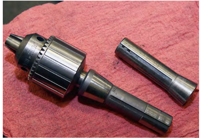
For drilling a chuck can be mounted to a collet and then inserted into the mill.
