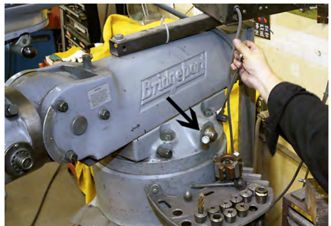
5) With the bolts shown here (there are a total of 4) you can slide the whole head assembly forward and back with the handle.
