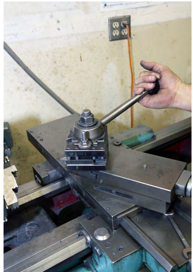
... twisting the handle shown here in a counter-clockwise direction. The nice thing about this is you have 5 or 6 different bits ready to drop on at a moment's notice.
