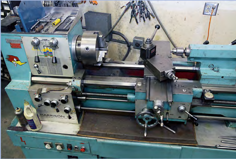
Your basic metal-cutting lathe with headstock, tailstock and tool support or carriage.
