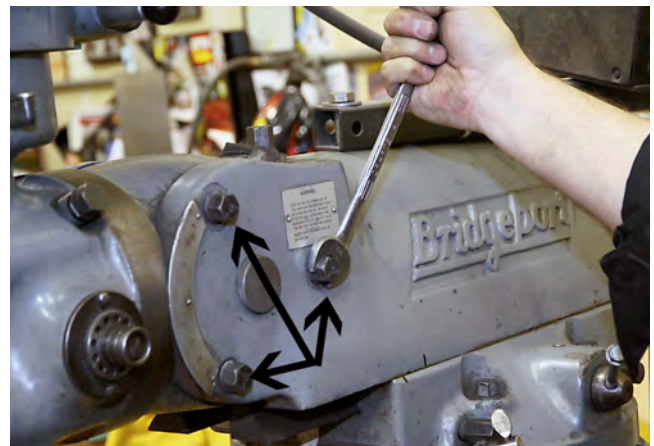
3) Or, you can loose the three bolt heads on the side of the mill...
