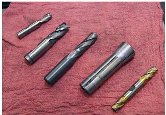
Some common tools include (top left to bottom right) a ball-end mill, a roughing or hogging mill, a 2-flute mill, a collet and a 4-flute mill.
