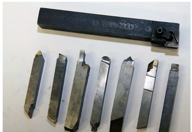
At Creative Metalworks, and most fabrication shops, tool blanks are shaped to fit the job at hand, these are just a few examples.
