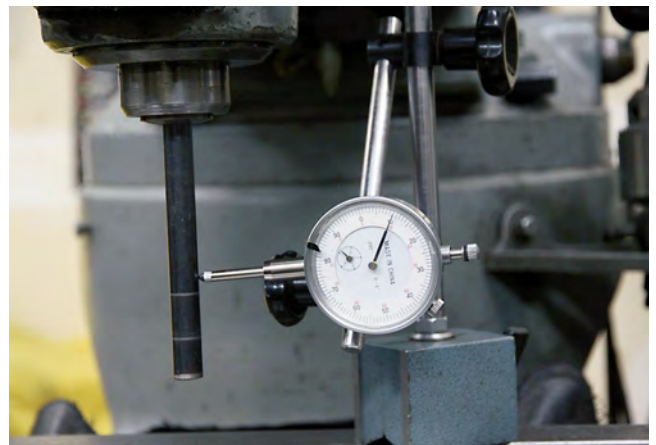
5) The reading on the dial indicator should remain constant as you raise the table. This Plan B method is much easier than the original Plan A.
