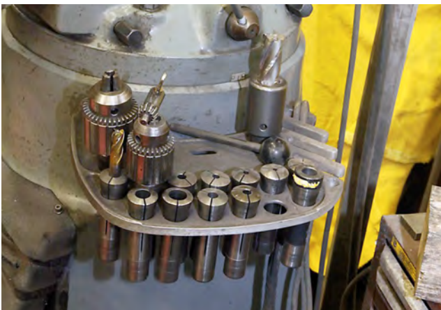
A variety of collets are needed for a variety of tools. Each ID matches the shaft OD of a particular tool.
