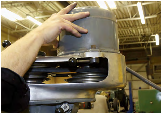
... put tension on the belt and lock the motor in place with the motor locknut handle.
